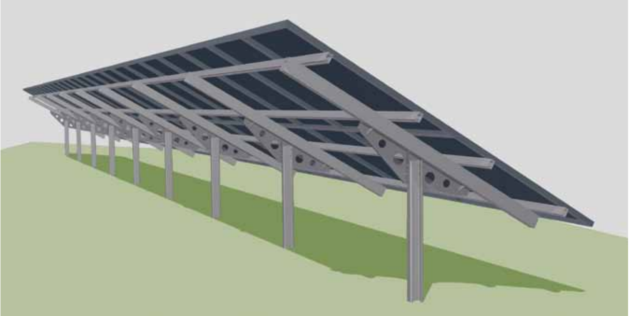
Planning example of an ground level with pile foundation, solar park Solsbor (Bulgaria)
